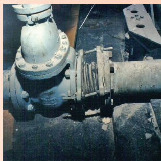
Teflon Bellows Failure
